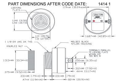
NOTE A: TERMINALS-.032 BRASS TIN PLATED, TAPPED FOR #6-32 SCREW. TWO #6-32 NICKEL PLATED BRASS SCREWS INCLUDED. WILL ACCEPT 1/4' QUICK CONNECT. TE B: MOUNTING- REMOVE BLACK PLASTIC NUT AND INSERT THREADED FRONT THROUGH 1.25° HOLE PUNCHED IN PANEL, IF DRIENTATION IS NEEDED, NOTE LOCKING FLATS ON DRAWING, SCREW NUT BACK ON. DO NOT OVERTIGHTEN.
