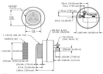
NOTE A: TERMINALS-032 BRASS TIN PLATED, TAPPED FOR #6-32 SCREW. TVD #6-32 NICKEL PLATED BRASS SCREWS INCLUDED. WILL ACCEPT 1/4\* QUICK CONNECT. NOTE B: MOUNTING- REMOVE BLACK PLASTIC NUT AND INSERT THREADED FRONT THROUGH 1.25' HOLE PUNCHED IN PANEL, IF DRIENTATION IS NEEDED, NOTE LOCKING FLATS ON DRAWING, SCREW NUT BACK ON. DO NOT OVERTIGHTEN.
